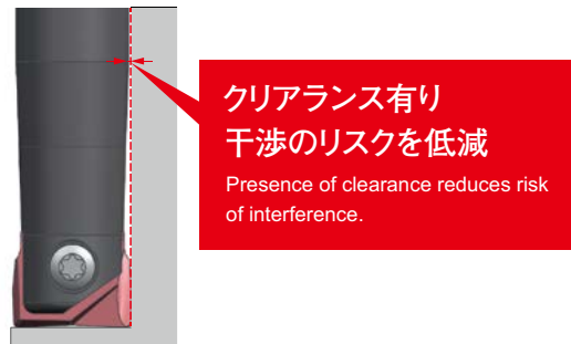
シャンク+1mm径インサート装着時 When insert with diameter +1mm larger than shank diameter is mounted.
